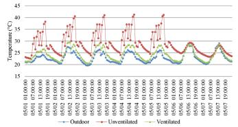
Figure 3. Thermal behavior - coffee processing plant - first floor - first week
