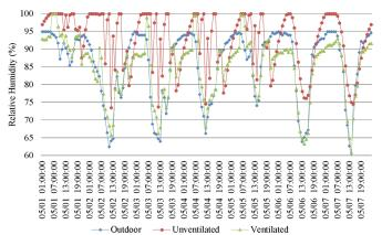
Figure 4. Relative humidity air - coffee processing plant - first floor - first week
