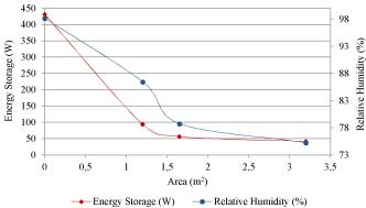
Figure 7. Energy balance and relative humidity for different openings for natural ventilation
